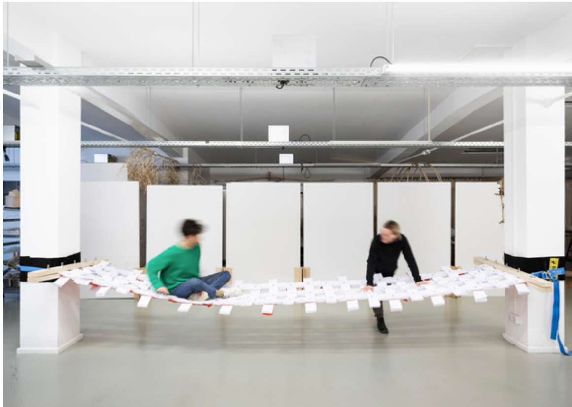
Hanging paper bridge made of approximately ten thousand A4 sheets held together by friction. Design and research: Lorenzo Guiducci, Maxie Schneider, Jojo Shone and Christiane Sauer
