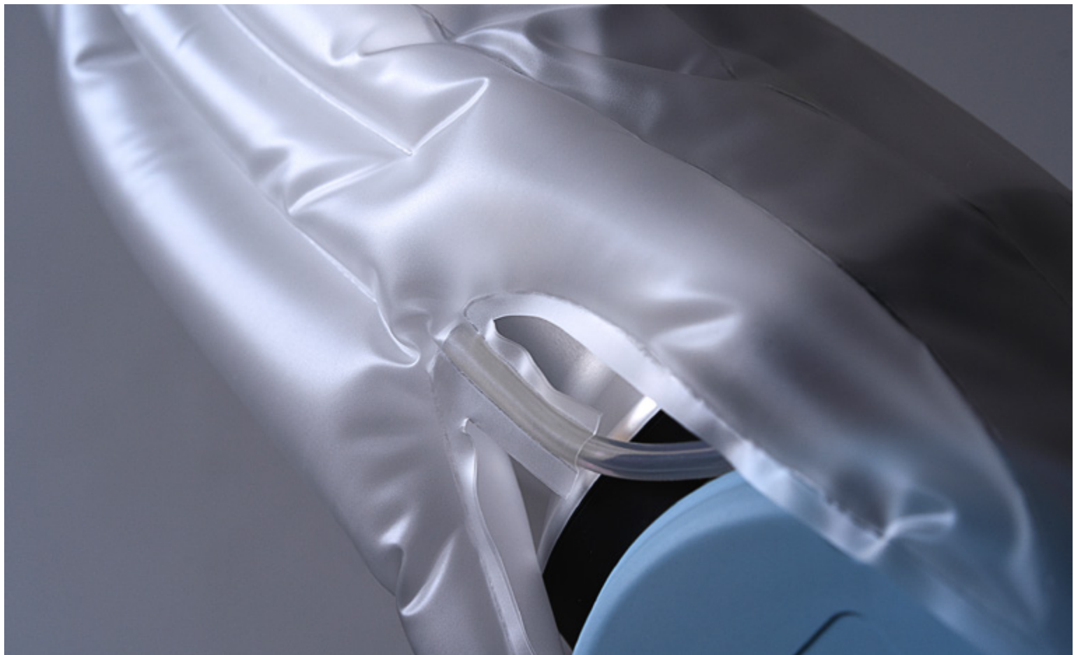
Pneumatic membrane as sensitive skin for a UR5. Photo: Anna Schaeffner
